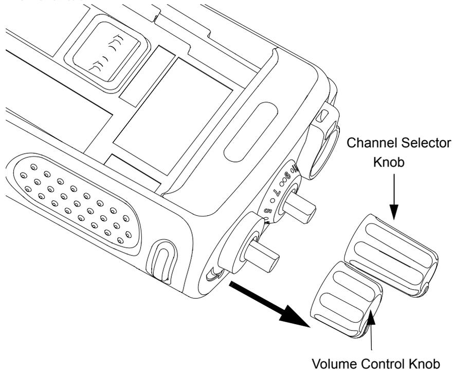
Figure 5-2. Channel Selector and Volume Knob removal.
