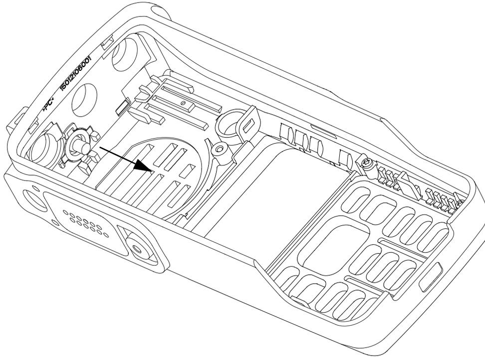
Figure 5-11. Emergency Button disassembly for Full Keypad Model
