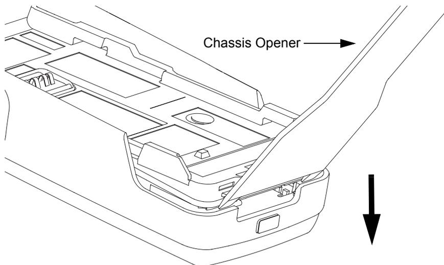
*Figure 5-4. Chassis removal*
