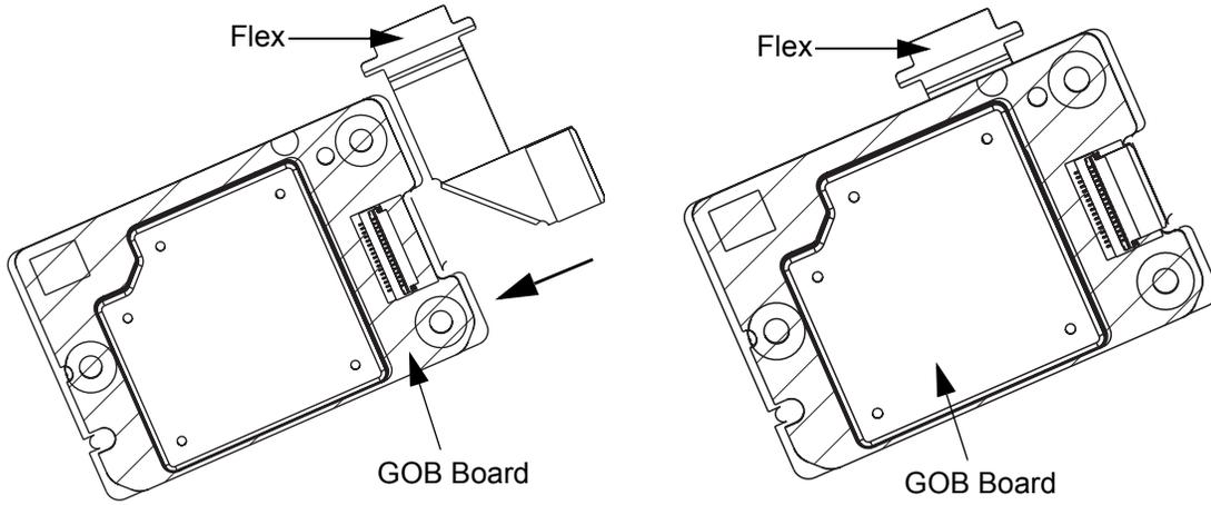
4. Insert the option board with the motherboard into the chassis as shown below.
