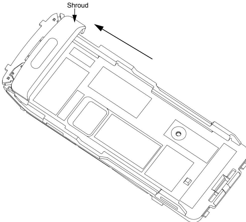
Figure 5-21. Chassis reassembly
