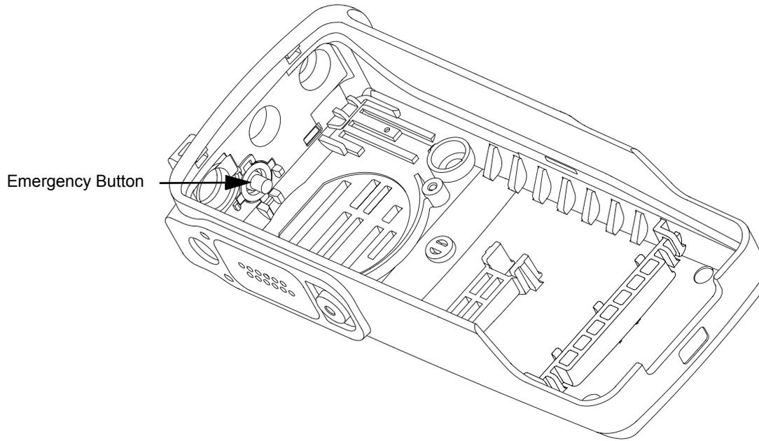
Figure 5-14. Emergency Button reassembly for Non Keypad
