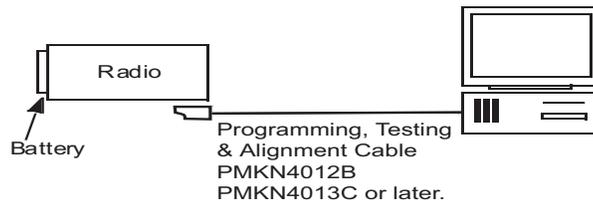
Figure 4-1. CPS Programming Setup
