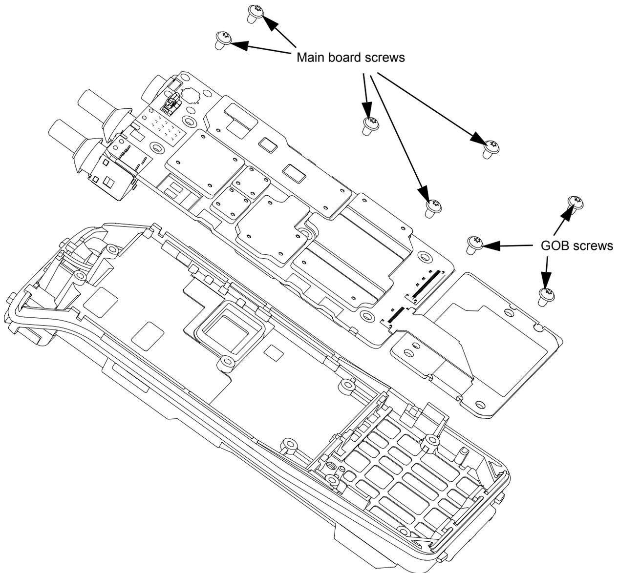
*Figure 5-19. Chassis reassembly*
