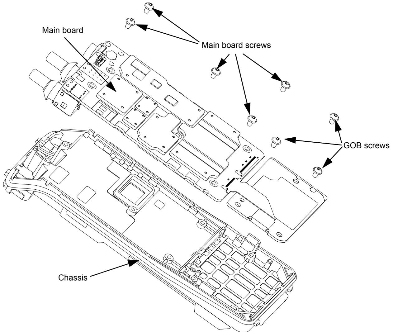
Figure 5-6. Chassis disassembly
