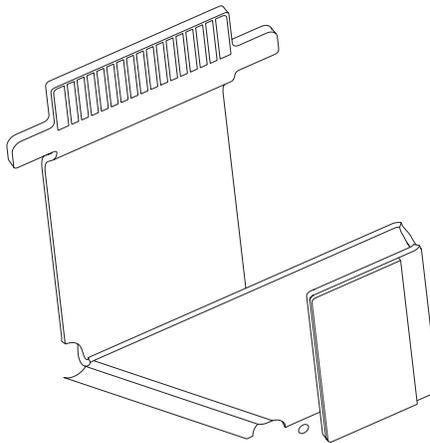
3. Gently lift the connector flap of the option board and connect the option board flex cable. Gently close the flap.
