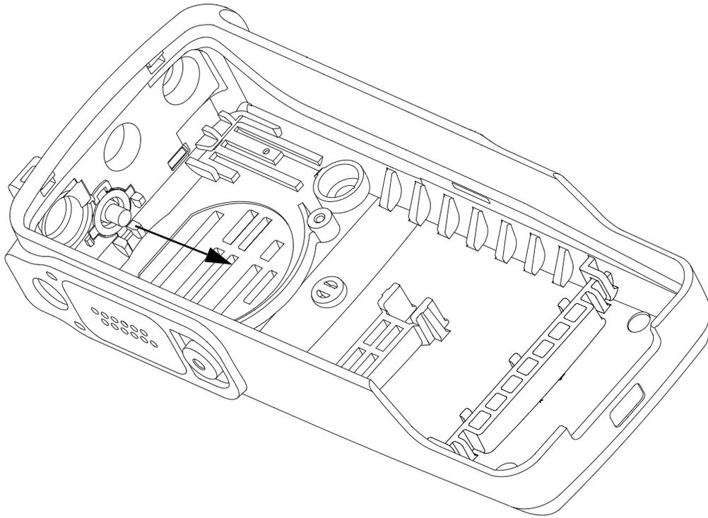
*Figure 5-12. Emergency Button disassembly for Non Keypad Model*
