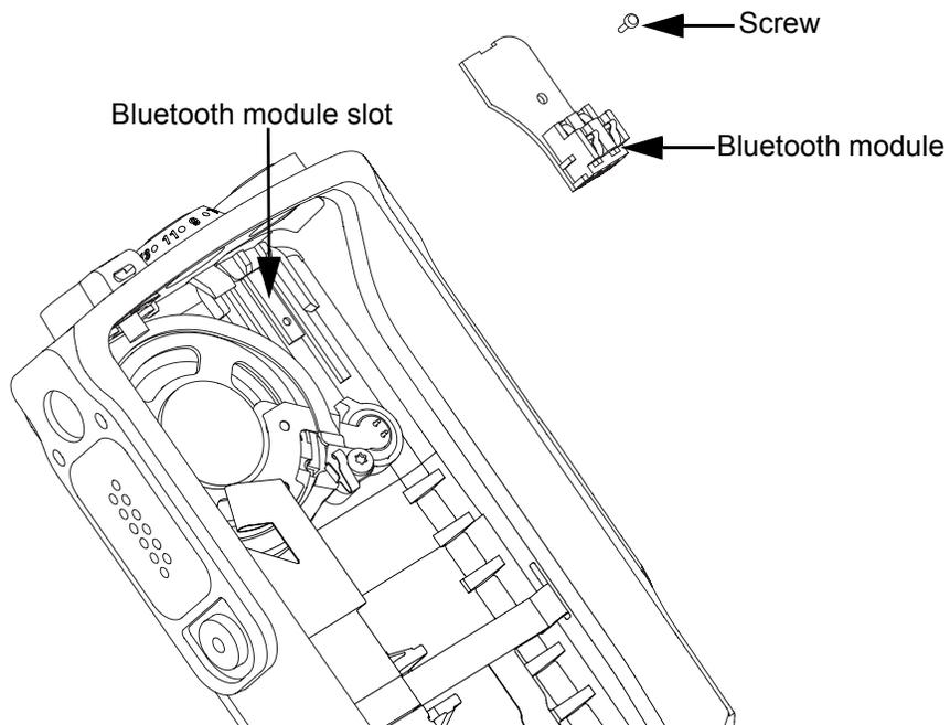
Figure 5-25. Bluetooth reassembly for Non Keypad
