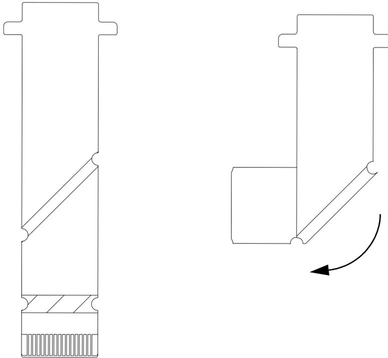
2. Peel the adhesive strip off from the spacer supplied and affix the spacer to the bottom side of the option board where marked.
