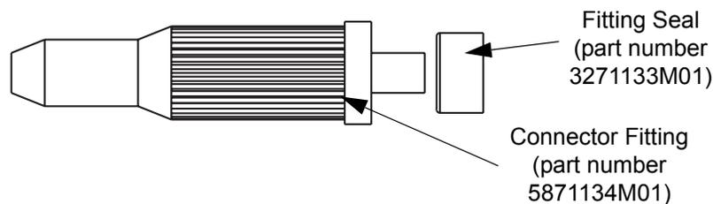
Figure 5-26. Connector Fitting - Fitting Seal Pump Connector
