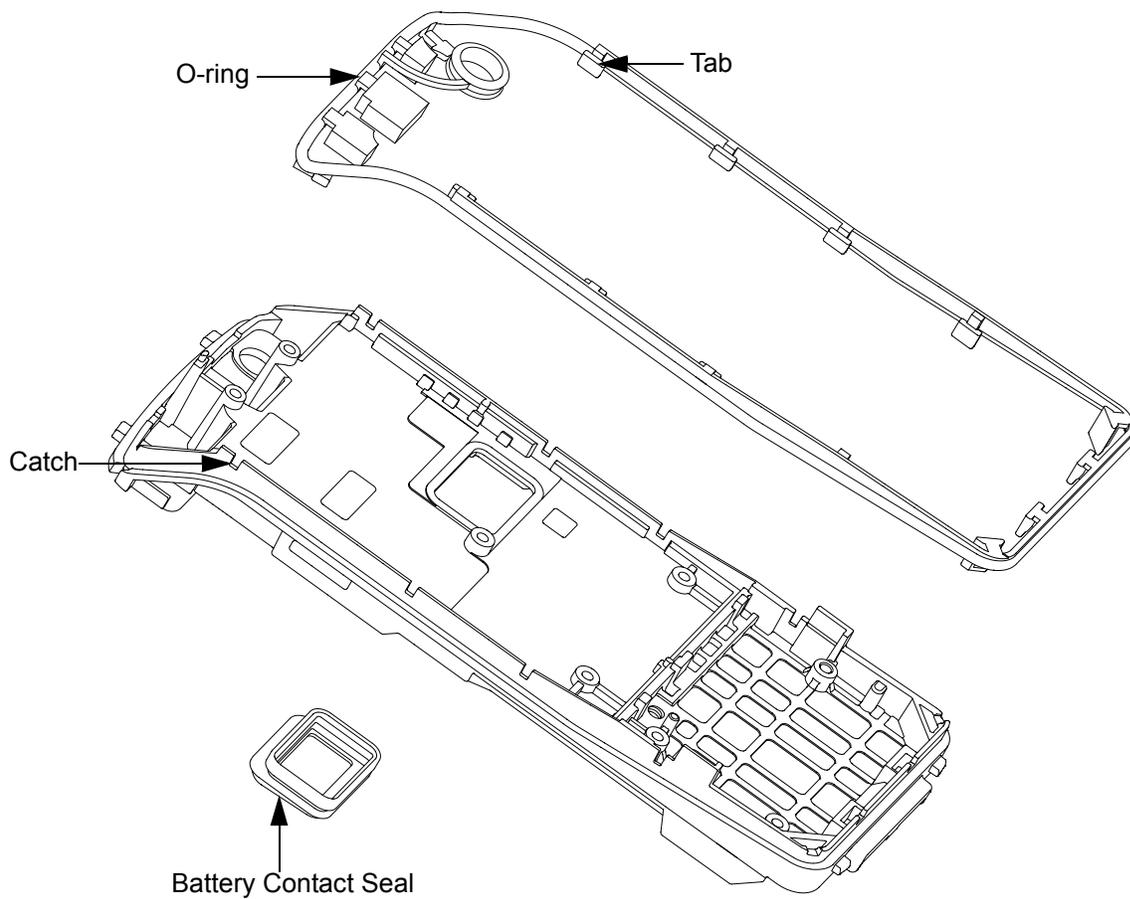
Figure 5-7. O-ring removal
