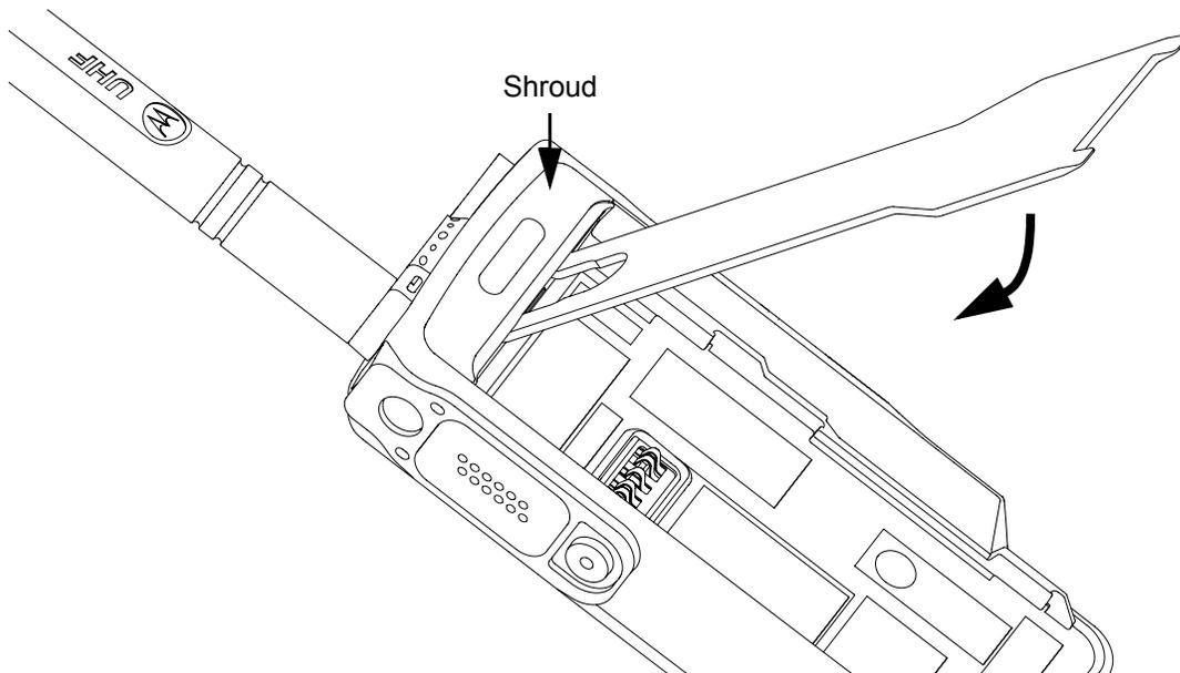
*Figure 5-3. Shroud removal*
